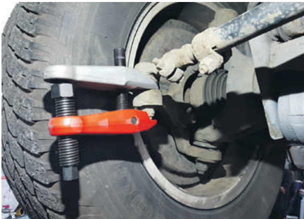
Audi - demontage spoorstangkop
